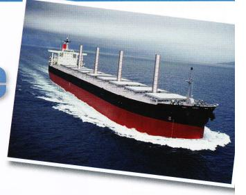
system, that converts wind into forward thrust aboard a ship, is an innovative and updated form of technology first introduced to the shipping industry in the 1920's. Described as a mechanical sail, the Magnuss VOSS utilises the Magnus Effect, a principle stating that a rotating cylinder in a wind stream produces a force perpendicular to the wind direction. Aboard a ship this effect can generate up to 80,000lbs of thrust, and in turn reduce the need for conventional fuel.
